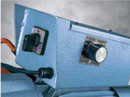
Variable Speed Control (Not Available on NF or 275 series) Recommended for cutting multiple shapes, sizes, and thicknesses. RPM can be fine-tuned to achieve optimum blade speed for each application and extend blade life.
